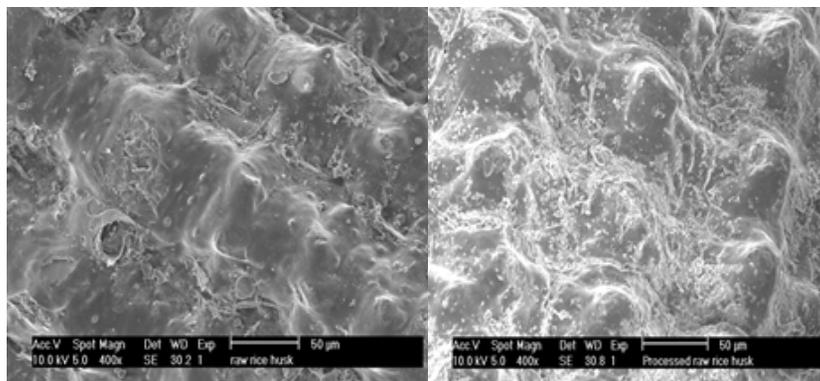
Fig. 4. RRH - SEM analysis of adsorbent (a) before and (b) after adsorption process.
