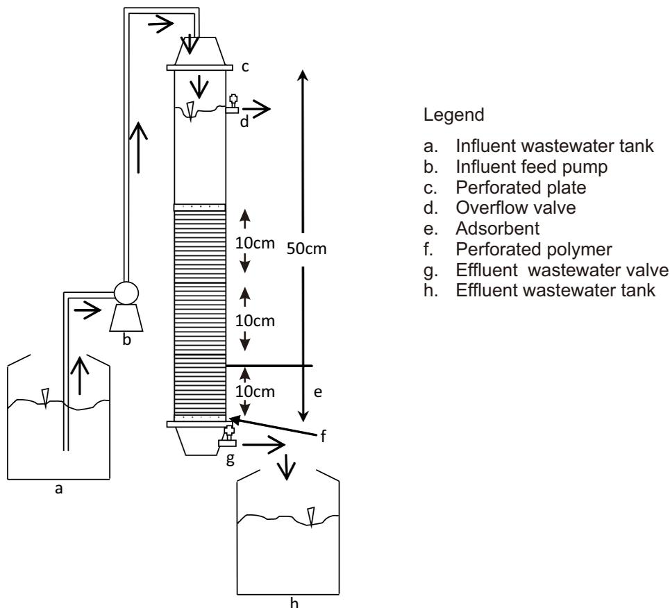
Figure 1. Schematic diagram of experimental setup for column studies
