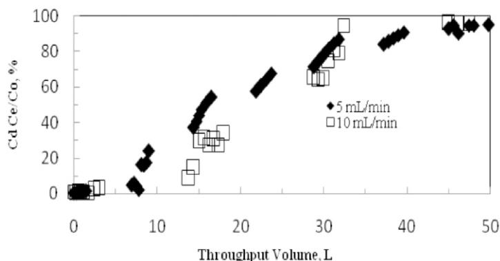
Fig.5. The experimental breakthrough curves for adsorption of cadmium from landfill leachate onto rice husk packed bed column at as a function of throughput volume in different flow rate.
